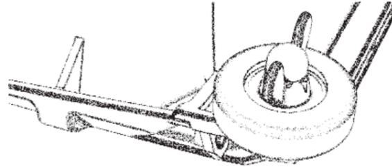
Fig.b-3 Left guide wheel installation completion diagram
