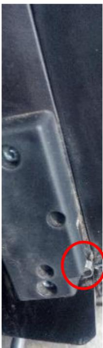
Fig.33-3 The switch rocker arm is fully closed
