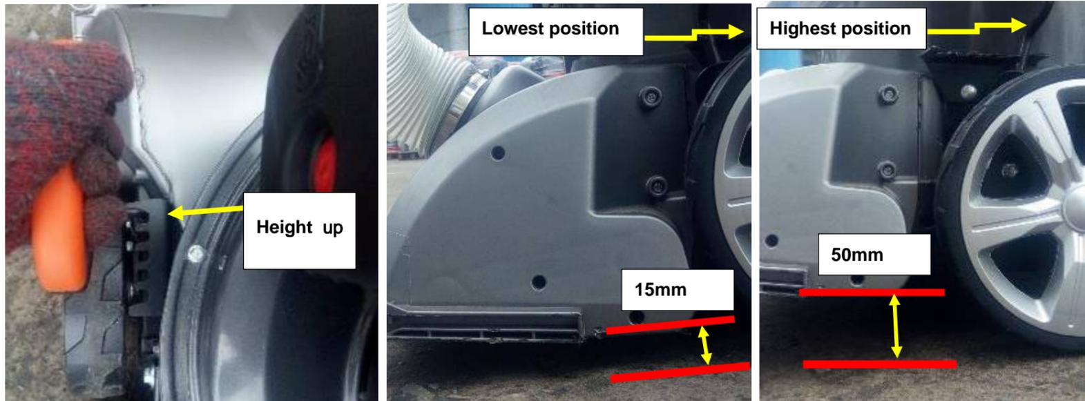
Fig.19-1 Pull out the handle
