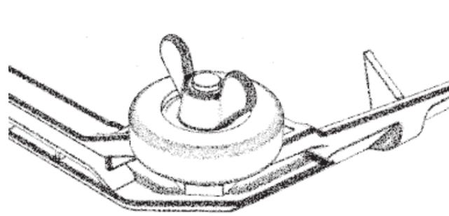
Fig.b-2 Right guide wheel installation completion diagram
