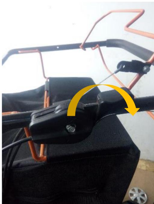
Fig.38 Engine Stop Throttle Control Position
