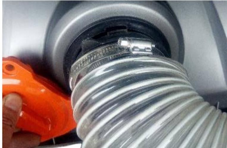
Fig.12-2 Insert hose connector
