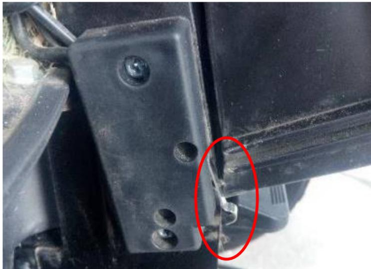
Fig.14-1 Switch rocker- Open position
