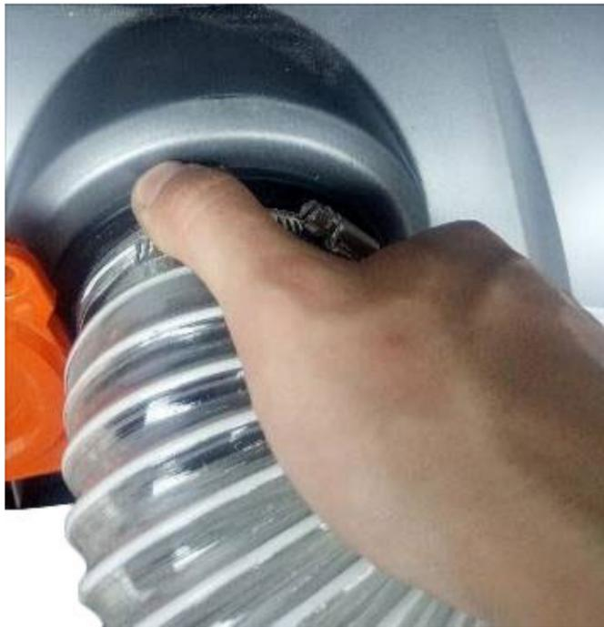
Fig.12-3 Screw the interface
