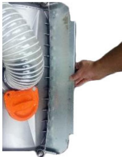
Fig.30-1 Insert baffle
