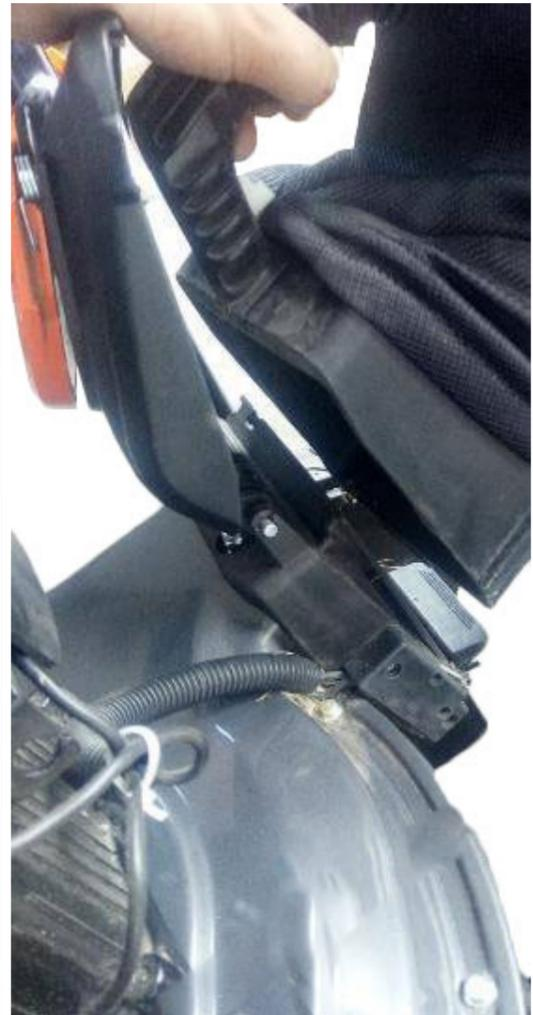
Fig.10-6 Insert back cover bracket
