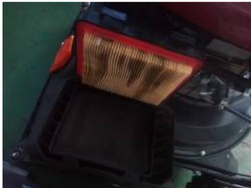
Fig.40-1 Open the air filter side cover
