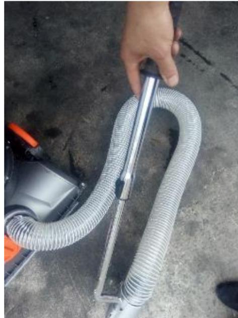
Fig.32-2 Adjust the telescopic height
