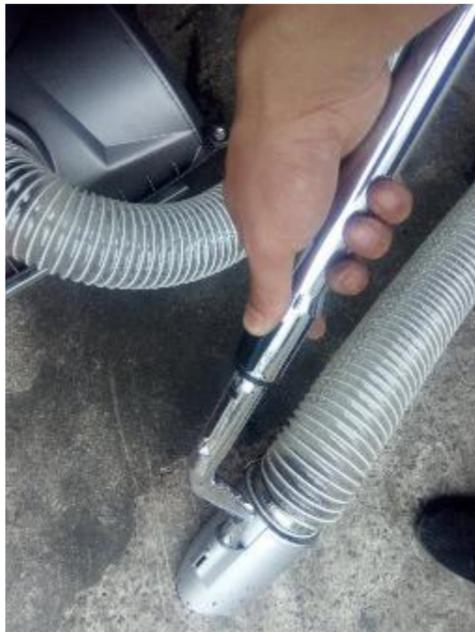
Fig.32-1 Push open the lock
