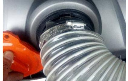
Fig.12-2 Insert hose connector
