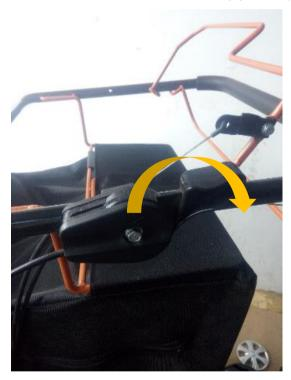
Fig.38 Engine Stop Throttle Control Position
