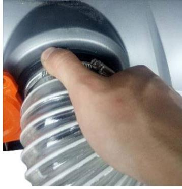
Fig.12-3 Screw the interface
