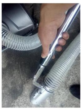
Fig.32-1 Push open the lock
