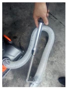
Fig.32-2 Adjust the telescopic height
