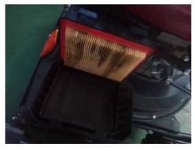
Fig.40-1 Open the air filter side cover
